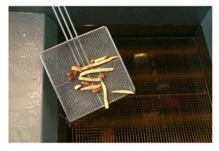
Prior to filtering, skim any large debris from oil in frypot.
